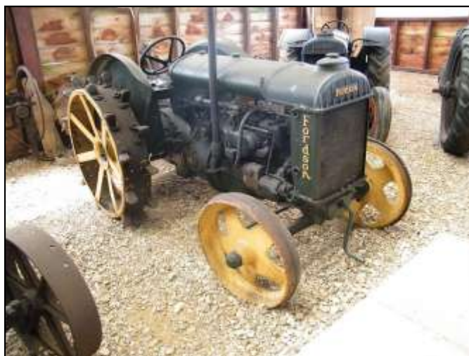
A 1944 Fordson 'Standard' Tractor with 'spade lug' rear wheels Image Source © austin7nut via http://www.flickr.com
